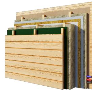
Section of the external walls with an internal drywall finish.
